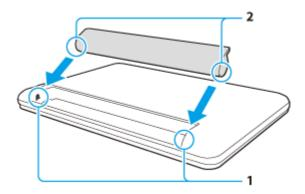
**4.** Turn the battery pack in the direction of the arrow and push the battery pack down into the compartment until it clicks into place.
